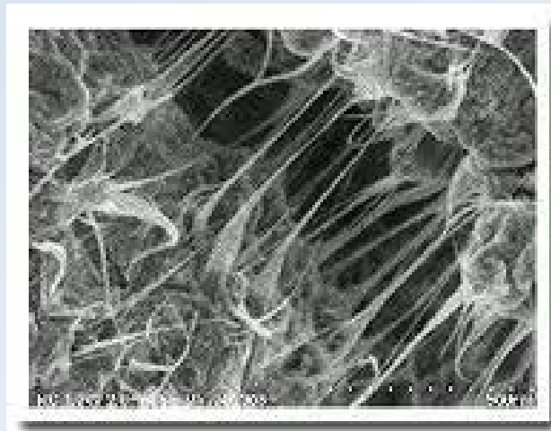
Crack bridging by CNTs
